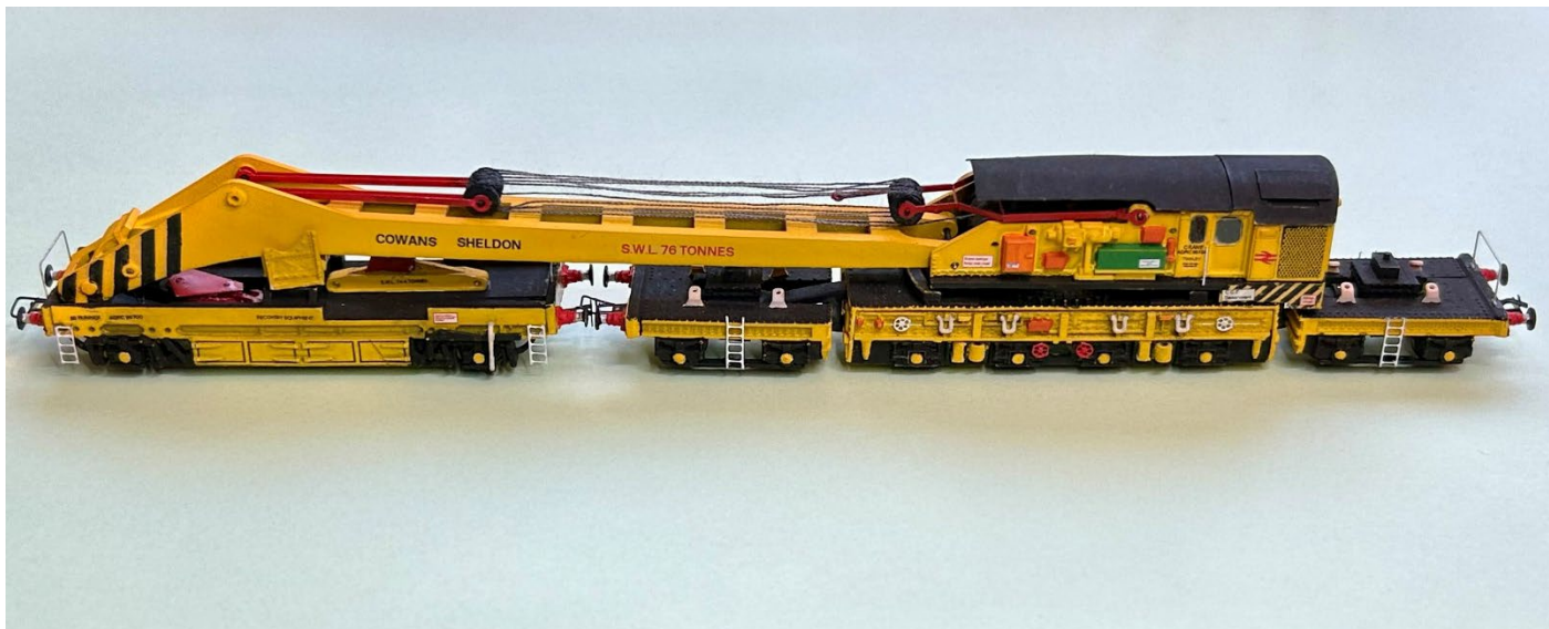
01 – Cowans Sheldon 76tonne Crane kit built and converted with 2mm scale wheels.
