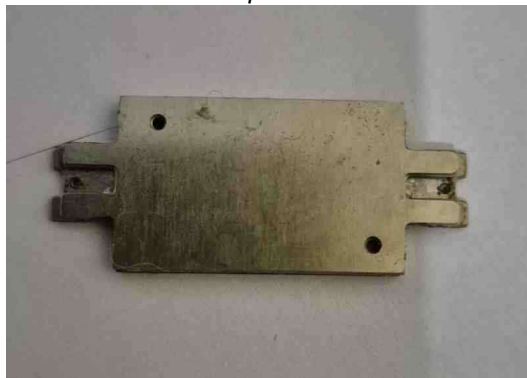
Bottom view - one slot is 1.75mm wide and the other slot is 2.05mm wide
